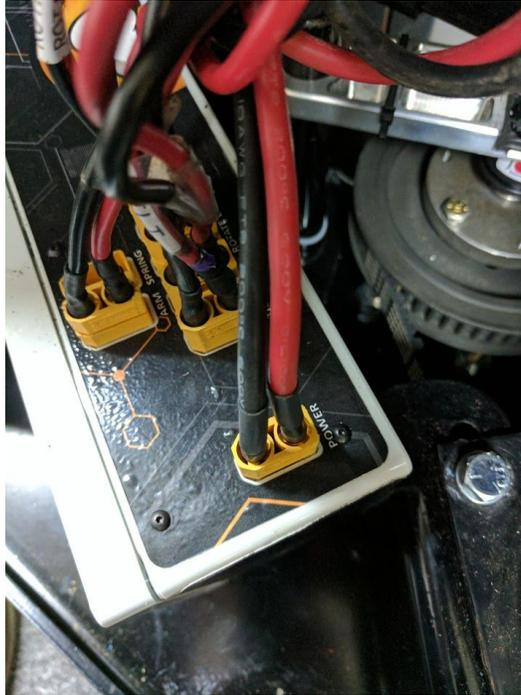
2. Make sure no wires are hanging in the center of the machine. Loose wires can easily get caught in the center pulley. All loose wires must be secured to the housing.
