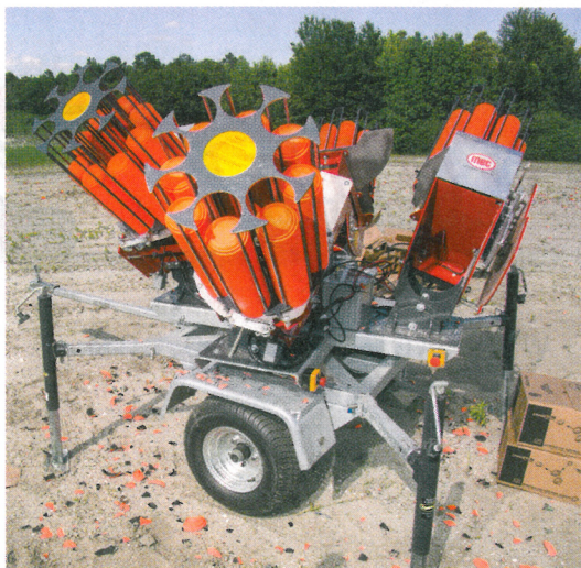
While spinning 360 degrees, the Quad by Crazy Quail can throw up to 160 targets per minute in any direction by wireless remote.
